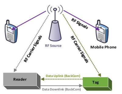
Since the TV or other nearby signals already have information on them, to avoid data overlapping between original and modulated signals, the passive tags transmit their data by reflecting the signals at a smaller bit rate than the surrounding radio waves rate. Afterwards, the receiver can differentiate among both signals by taking their mean value.
